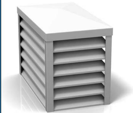
Suitable for sizes up to 1500mm x 1500mm. Comprising louvres on four sides with aluminium corner posts and acoustically lined aluminium pyramid roof. For larger sizes an aluminium base angle frame and acoustically lined gable roof are available. Sectionalised where necessary for assembly on site
