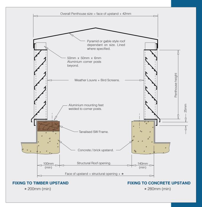
Bird or vermin guard galvanised mesh fixed to the rear of the louvre section. = BS
