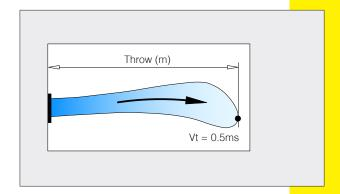
Additional factors can be applied to correct for other terminal velocities and temperature differentials. Jet drops can also be estimated from the nomogram on page 10 of **PART L**. Acoustic data is presented in terms of NR levels based on a room absorbtion factor of 8dB.
