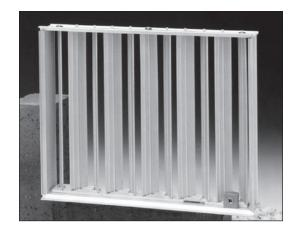
The standard method of adjustment is by a removable key through the grille face, but lever and right angle type operators, together with fusible fire links, can also be supplied. Where necessary, the dampers incorporate end closure plates to provide an effective seal in the closed position.
