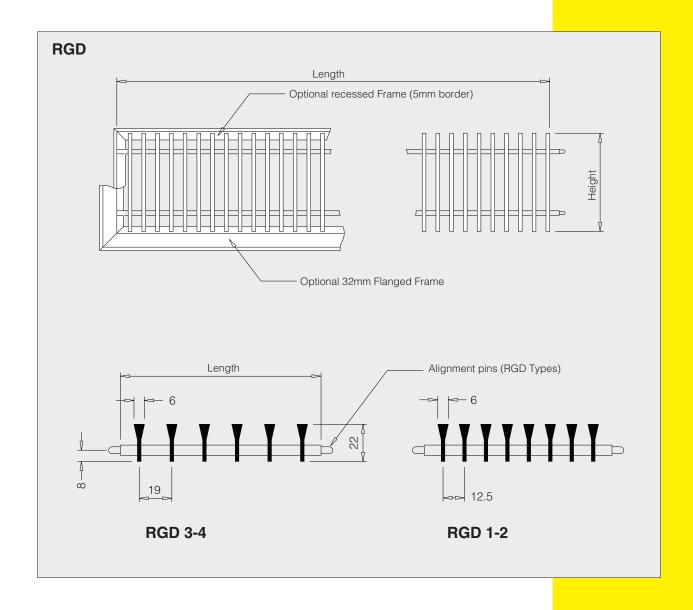
RIGIDCORE GRILLES should **NOT** be used for pedestrian traffic or heavy point loads. Designed for fitting under glazing etc., and only occasional foot traffic.
