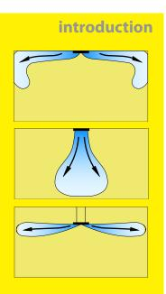
The MRA range of circular diffusers are high air capacity terminals specifically designed to suit applications such as atria, auditoria or industrial premises. The core position is adjustable on a central screw thread giving conventional horizontal diffusion with exposed duct or ceiling mounted installations, or a progressively adjustable vertical projection setting for spot cooling and heating applications.
