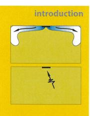
The F45 <sub>-</sub> louvre style ceiling diffuser offers an alternative form of continuous air distribution system for variable air volume or fan coil applications.
