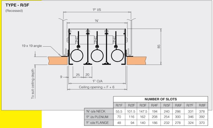
Note: inside Plenum length add 10mm when using end caps.
