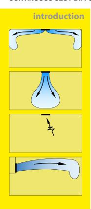
The Flowline diffuser has been specifically developed to meet requirements for an aerodynamically efficient continuous slot air distribution system. The unique design of the deflection tube produces both low noise and low pressure losses, making it suitable for use with variable air volume, fan coil or induction systems.
