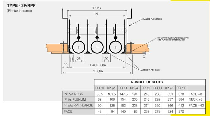
Note: inside Plenum length add 10mm when using end caps.
