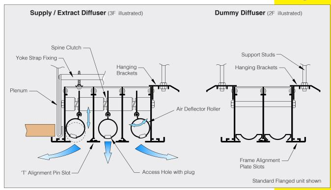
Lateral and vertical adjustment of the deflection tubes provides full directional jet control and discharge velocity regulation. The aerodynamic profile of the tube also gives the Flowline diffuser a wide dynamic flow range, making it particularly suitable for variable air volume application.
