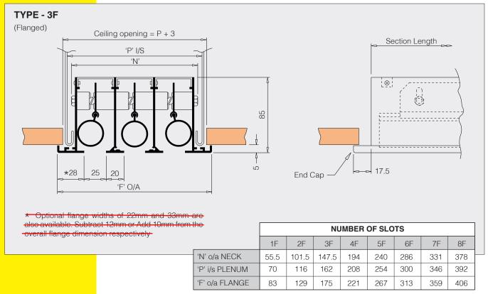
Note: inside Plenum length add 6mm when using end caps.
