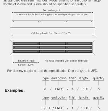
When ordering corner sections, state the number of slots required, the inside lengths A and B, the angle and the finish designation code.
